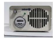
Check for the "corona discharge" in the front of the machine through the slots. You should see a vertical "black light" line (purple) that is straight with no spotting. If this is not the case, the titanium plates need to be cleaned again. (If you cannot see the black light, plug the machine in a darker area of the room.) Sighting the straight line is an indication that your machine is running at optimum performance.
